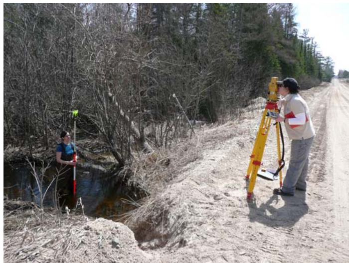
NRCS Engineer, Andrea Paladino, and Huron Pines AmeriCorps member, Casey Ressler, gather survey information for the road crossing site design.
